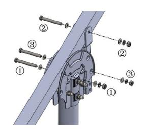
4) Fasten the Steel Cap Assembly to Pipe with M14\*150, M14\*110 Hex Bolt, keep the Rectangular Tube-Master parallel to the south-north by adjust the Steel Cap Assembly.
