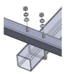
2) Preassemble the Cross Connection Clamp at the Rectangular Tube-Master with M8\*70 hex bolts, plain washer 8, spring washer 8, and M8 nut as shown in the figure on the right.
