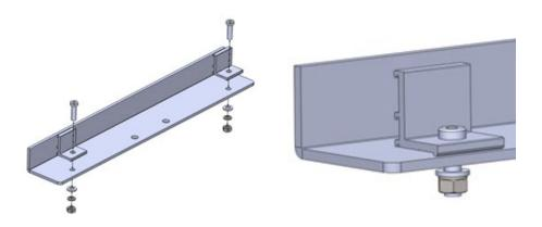
2) Connect the Angle Bracket to Rectangular Tube-Master with 8pcs U bolts, 16pcs M10 nuts, 16pcs spring washer, 16pcs washer as shown in the figure below.
